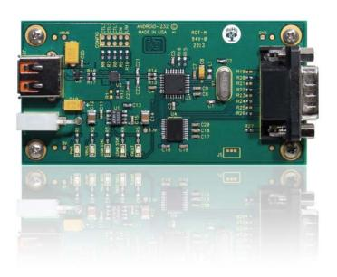
RS-232 Serial Adapter for Android Devices Features Industrial Temperature Operation
