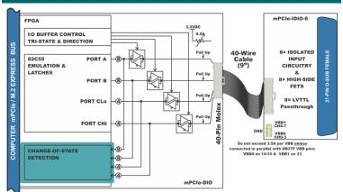
This manual applies to both the mPCle and M.2 cards listed on the cover page as these devices are register and functionally identical. This device consists of an M.2 or mPCle interface board that connects to a Mobile-ITX-sized, panel- or plate-mountable DB-37F Isolation Module via an included 9" cable.
