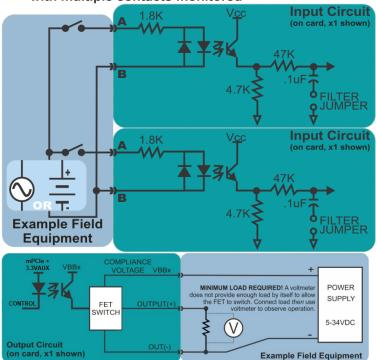
TB1 provides an alternate location for connecting VBB0 and VBB1 in parallel with the DB37F pins. You may find the screw terminals more convenient when sourcing power from inside your enclosure.
