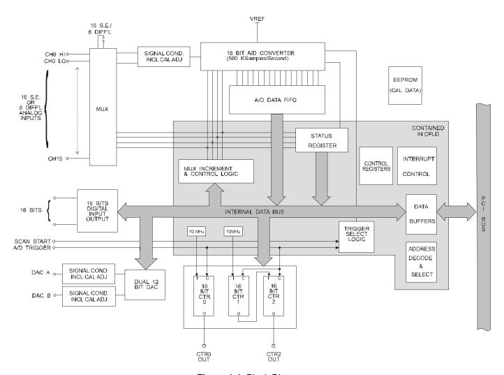
Figure 1-1: Block Diagram
