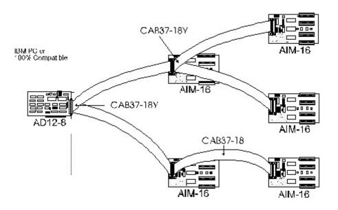
Figure 2-1: Use of CAB-37Y Cables
