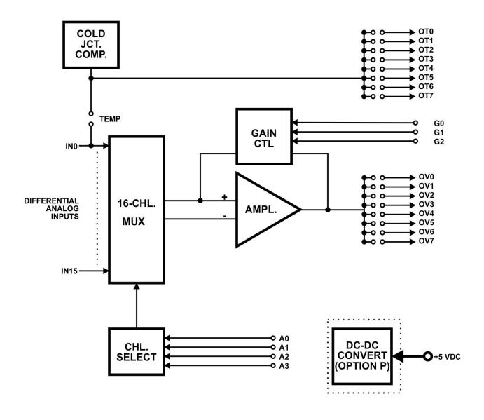
Figure 1-1: AIM-16 Block Diagram
